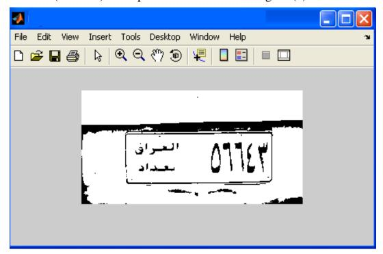
Figure (3): The Plate area segmented
