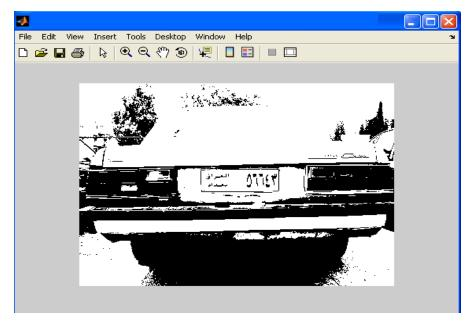
Figure (2): Thresholding image
