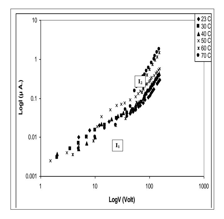
Fig. (4): The (log I-log V) characteristics at different temperatures.
