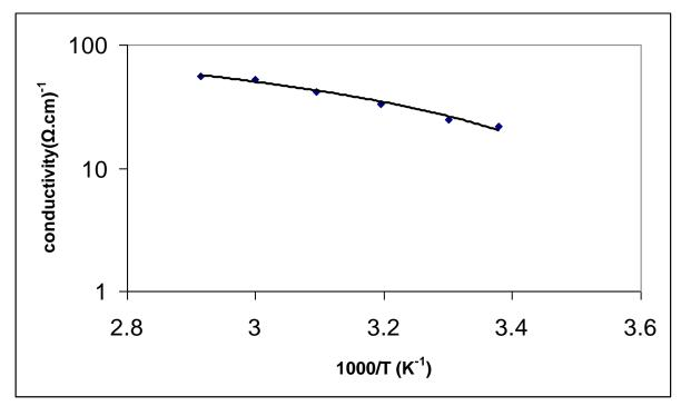
Fig. (6): The relation between  $(\log \sigma)$  and temperature.
