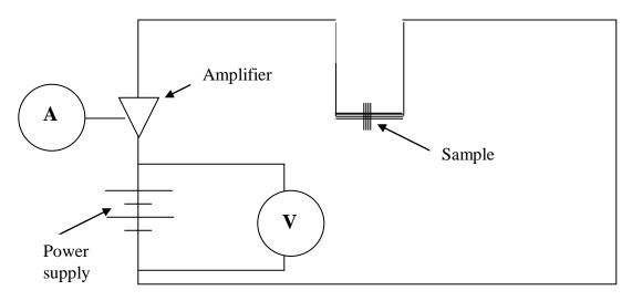
Fig. (1): The measurement circuit of (I-V) characteristic.
