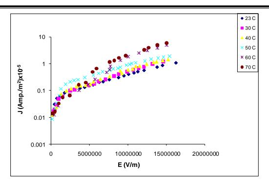
Fig.(7): the relation between(log J) and effective field strength
