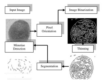
Figure (4): minutiae detection algorithm
