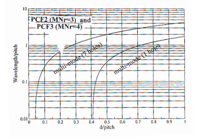
Fig. 8: Cut-off phase diagram for one and seven holes missing [21].
