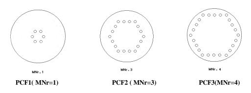
Fig. 2: Cross section of the proposed structure with core radius  $R_c = Nr \times \Lambda - d/2$
