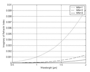
Fig. 5: Imaginary part of the effective index of the fundamental mode as a function of wavelength for the proposed structures.
