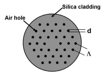
Fig. 1: A cross section diagram of a photonic crystal fiber.
