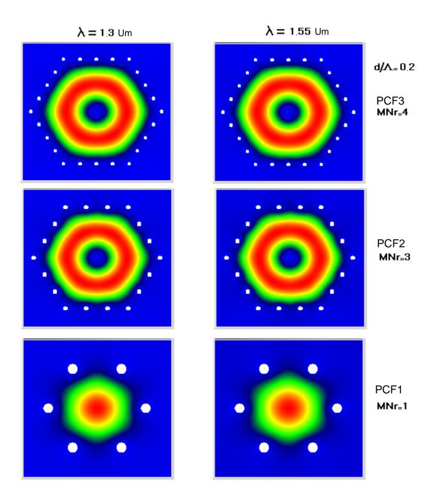
Fig. 9: The field distribution of the mode at communication wavelengths 1.3 & 1.55 $\mu$ m, all the proposed structures of relative air hole d/A = 0.2
