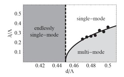
Fig.3. Cut-off phase diagram, the solid line separating the single and multi mode regimes for a fiber of one missing hole [12].
