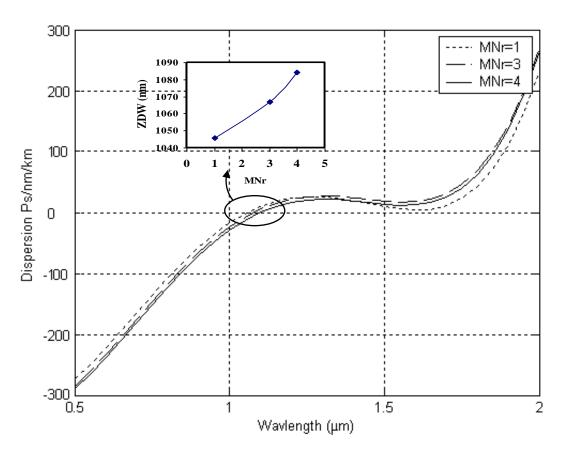
Fig.6. Computed dispersion as a function of wavelengths for a proposed PCFs.
