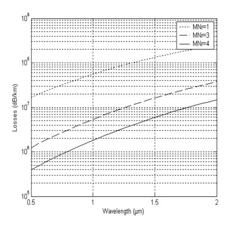
Fig. 7: Computed confinement losses as a function of wavelengths for proposed PCFs.
