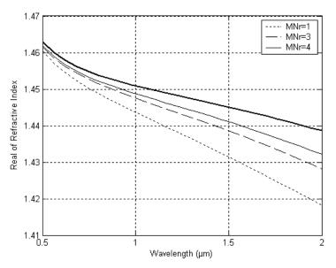
Fig. 4: Real part of the refractive index of the fundamental mode as a function of wavelength for the proposed structures, the bold line for silica.
