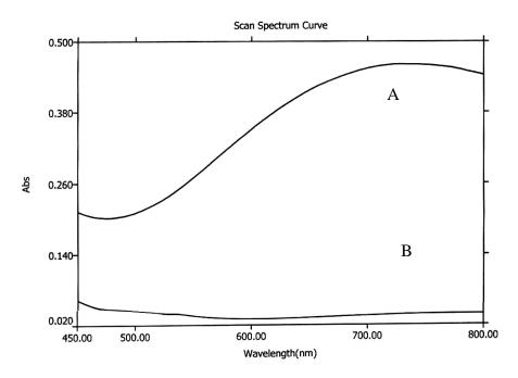
Fig. [1]: Absorption spectra of tolnaftate product against blank (A), with reagent blank against water (B) (tolnaftate taken 2 μg/25 ml)
