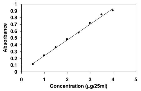
Fig [2]: calibration graph of tolnaftate. Accuracy and precision: The accuracy and precision of the method were established by analysing the pure drug at three different concentrations and seven determinations. The average recovery which is a measure of accuracy is 100.3% revealing high accuracy of the method. The relative standard deviation (RSD), which is an indicator of precision is less than 2.5% the results are cited in table [5].
