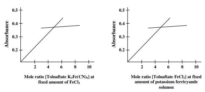
Fig. [3] : Molar ratio method of toluaftate-FeCl<sub>3</sub>-K<sub>3</sub>Fe(CN)<sub>6</sub> Effect of interferences:
