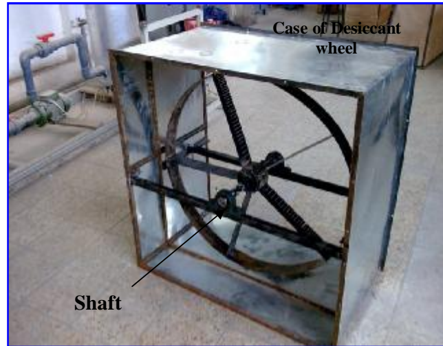
Figure (5) Case of desiccant wheel
