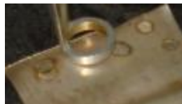
Figure (3) Silver drilled by 1064nm 1 st harmonic Nd:YAG laser at 1J
