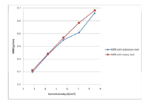
Figure (4) Effect of rotary action of tool on MRR compared with stationary tool.
