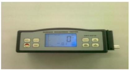
Figure (2) surface roughness device.
