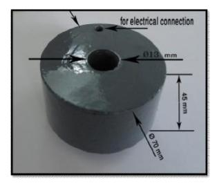
Figure (3) Workpiece being used in the experimental work
