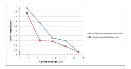
Figure (7) Ra with rotary and stationary tools at ]different current densities
