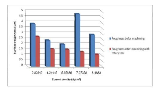
Figure (8) The differences in surface roughness before and after ECM machining in different current densities with rotational tool
