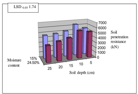
Figure(9): The relationship between the soil penetration resistance and soil depth for five pass on the soil surface.
