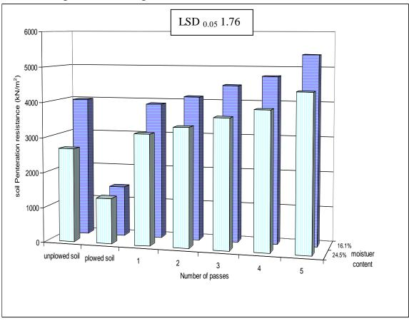
Figure (4): The soil penetration resistance versus the number of passes for two moisture content levels.
