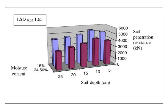
Figure(6): The relationship between the soil penetration resistance and soil depth for two passes on the soil surface.
