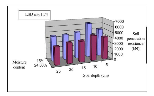
Figure(8): The relationship between the soil penetration resistance and soil depth for four pass on the soil surface.
