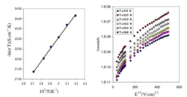
Figure(8):The relationship between  $-ln(\ \sigma \ T)$  and  $10^3/\ T$  .
