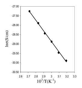
Figure(6): The relationship between  $ln\sigma(T)$  and  $10^3/T$ .
