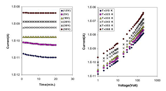
Figure(4):The relationship between current and time at different voltage (1.5-50V).
