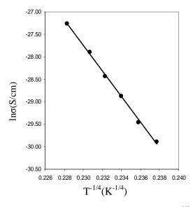
Figure(7):The relationship between  $In\sigma(T)$  and  $T^{-1/4}$ .
