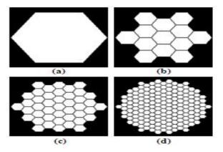
Figure (1) Segmented aperture:  $N_h$ = 1. b-  $N_h$ = 13. c-  $N_h$ = 43.d-  $N_h$ = 169.
