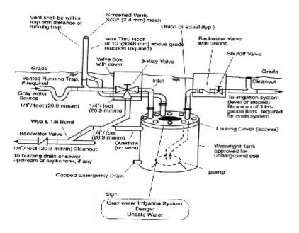
Figure (8) underground pumped system used for drip irrigation purposes.
