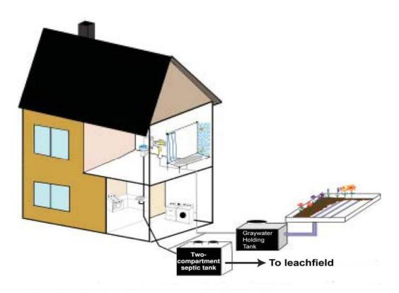
Figure (5) House diagram of separate black water and gray water plumbing systems.
