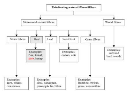
Figure (1) Classification of natural fibers which can be used as reinforcement of polymer [4].
