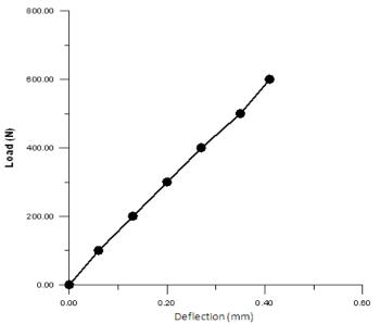
Figure (6)The load – displacement of epoxy matrix composite reinforced with 3 % wt okra fiber.
