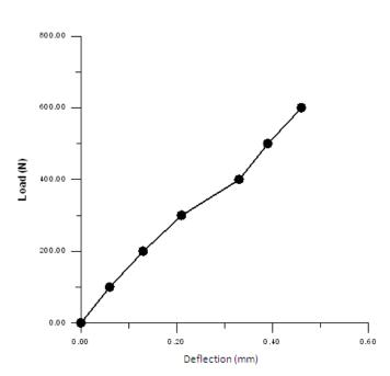
Figure (5)The load – displacement of epoxy matrix composite reinforced with 1 % wt okra fiber.
