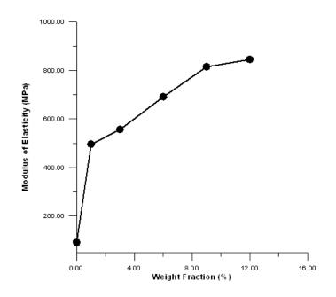
Figure (10) Effect of weight fraction of short okra natural fiber on modulus of elasticity of epoxy matrix composite.
