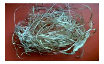
Figure (2)Extracted okra fibers.
