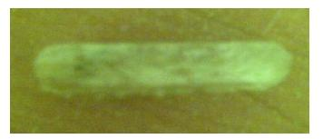
Figure (3)Impact test specimen of okra fabric reinforced epoxy composite.
