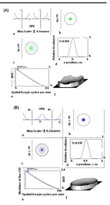
Figure (8) Characteristics curves of micro keplerian telescopic system with  $F_{\#}5$ , for (A)  $r_0=0.0mm_{(B)}r_0=0.04mmm$ , where in both A & B a) OPD at image plane, b) spot diagram at mid focusing plane, c) spot diagram at image plane, PSF with Strehl ratio S =0.968 in A & S=0.947 in B, e) MTF curve, f) wavefront map.
