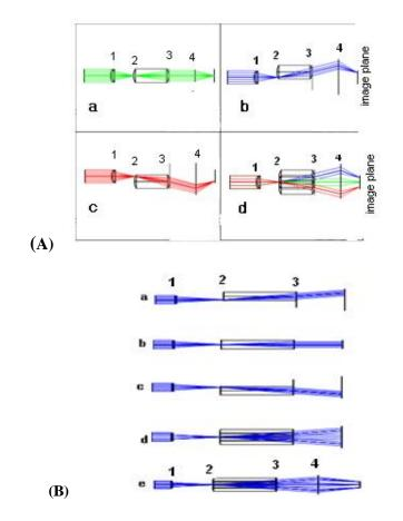
Figure (7) Designed Keplerian telescopic Afocal micro scanner system for maximum
