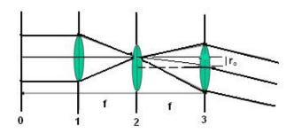
Figure( 6) Keplerian Afocal telescopic type scanner system 1-objective lens, 2-field lens, 3- eyepiece lens [ 8 ].
