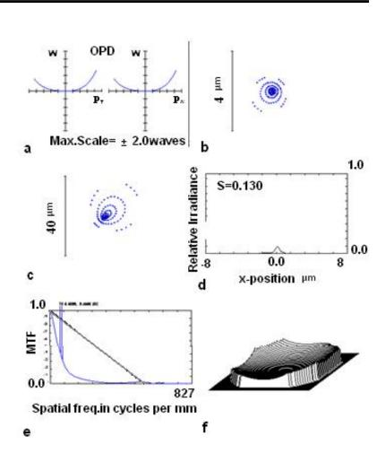
Figure (9) Characteristics curves of Keplerian micro telescopic system with  $F_{\#}$  1.5, for  $r_0$ =0.04mm, a) OPD at image plane, b) spot diagram at mid focusing plane, c) spot diagram at image plane, d) PSF with Strehl ratio=0.130, e) MTF curve, f) wavefront map.
