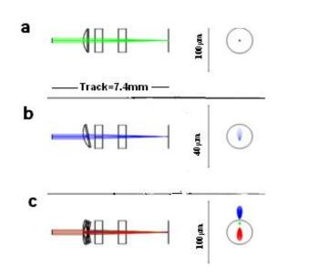
Figure (3) Layout of single aperture micro scanner(case 1, ENPD=0.3mm,  $\lambda = 1.064 \mu m$ ), a) at 0° tilt angle, b) at +11.5° tilt angle, c) at all tilt angles, on the right are shown spot diagrams at the image plane surrounded by the Airy disc.
