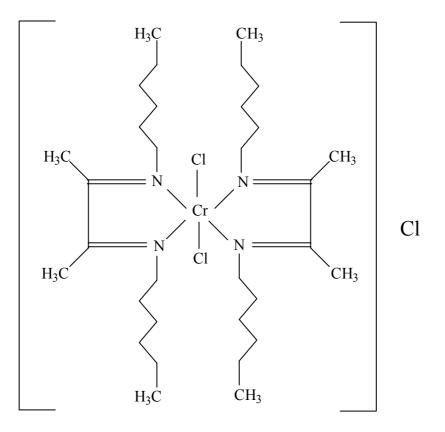
**Fig.1 : Suggested structure of the chromium(III) complex**
