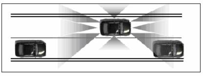
Figure(2): Car with front and back radars networks
