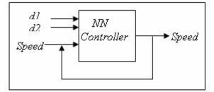
Figure(4): NN controller for straight running
