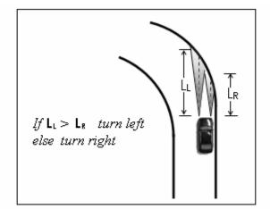
Figure (6): Nerocontroller system turn car to left depending on the  $L_L$  and  $R_R$  distances
