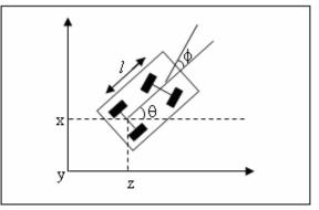
Figure(7): The stern angle is ranged between  $\pm 60^{\circ}$
