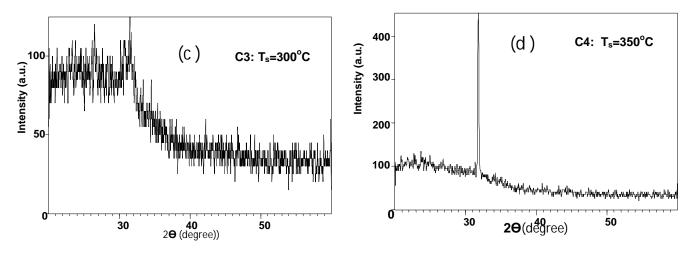
Fig.(1):XRD pattern of SnS thin films prepared at different Sub. Temp .
