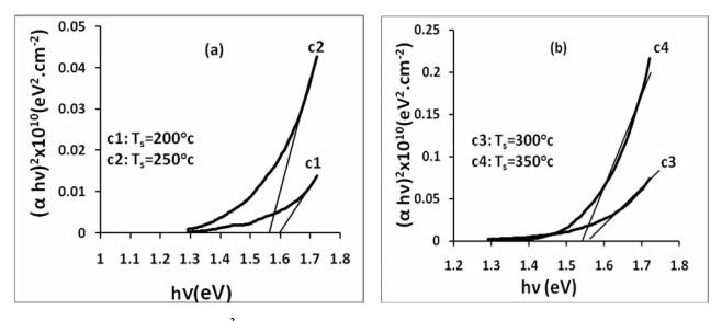
Fig.(7): Plot of  $(\alpha hv)^2$  as a function of photon energy (hv) for SnS thin films.
