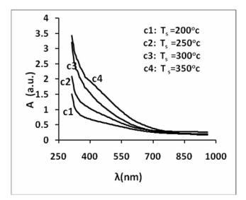
Fig.(4):Spectral behavior of Absorbance for SnS thin films prepared at different
