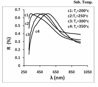
Fig.(5):Spectral behavior of Reflectance for SnS
