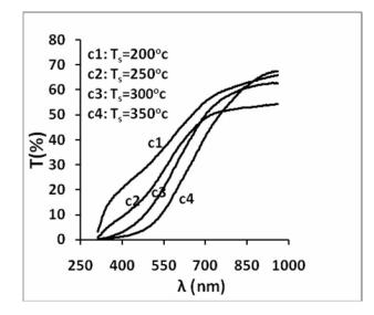
Fig.(3): Optical Transmittance spectrum for SnS thin films prepared at different Sub. Temp.
