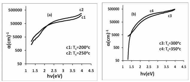
Fig.(6):Absorption Coefficient ( $\alpha$ ) for SnS thin films prepared at different
