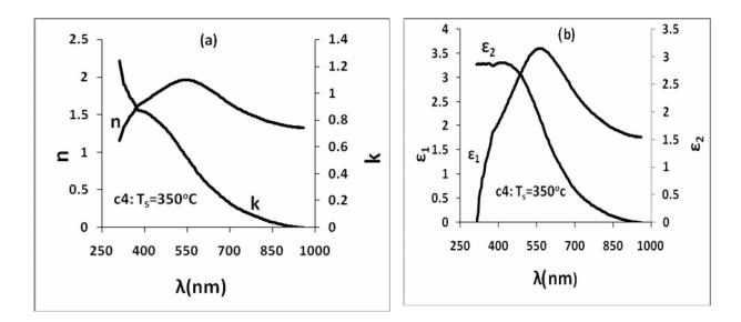
Fig.(8): Spectral behavior of (a): Refractive Index (n)and Extinction Coefficient (k).
