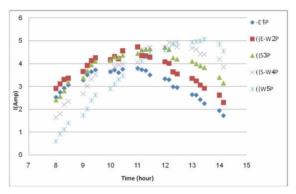
Fig (7) shows the output solar panels (current) with the time
