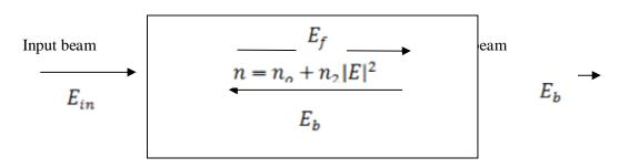
Fig(1) A nonlinear Fabry-Perot cavity
