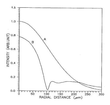
Fig (3) The normalized intensity profile : A)at the input, B) the transmitted at the switch up point.
