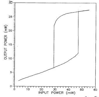
Fig (2) The transmitted power versus the input one  $\lambda = 5.5 \,\mu m$ ,
