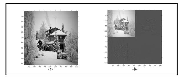
Figure 3: An image with its DWT (a)The image, (b)Its 1\_Level 2D\_DWT 56
