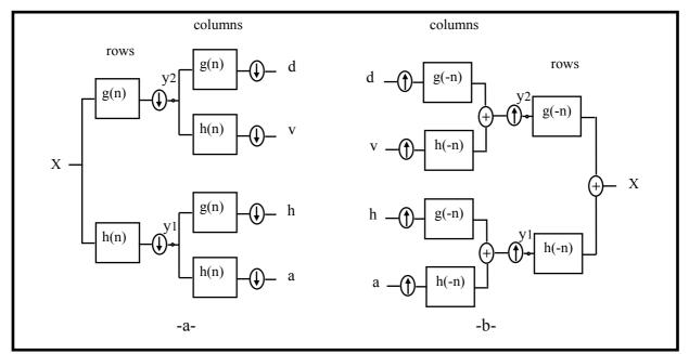
Figure 1 :1\_Level 2D\_DWT (a)Decomposition , (b)Reconstruction
