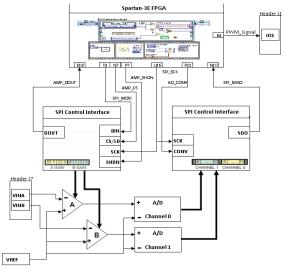
Figure 2. Block Diagram of the complete system implemented on Spartan-3E kit
