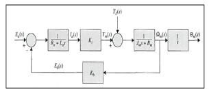
Figure 8. diagram of a D.C. motor system
