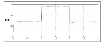
Figure 9. System response to the sudden change of speed reference
