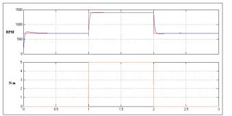
Figure 12. System response to the sudden change of speed reference and load
