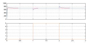
Figure 10. System response to sudden change of load at 700 rpm constant speed
