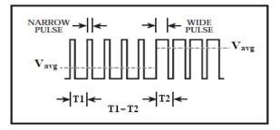
Figure 5. Pulse width determines average voltage with fixed period
