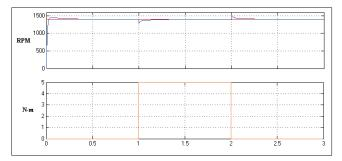
Figure 11. System response to sudden change of load at 1400 rpm constant speed
