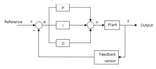
Figure 1. Closed loop PID Controller
