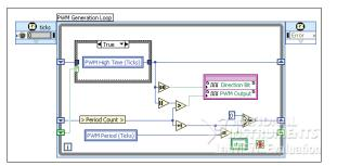
Figure 6. PWM signal generation block diagram
