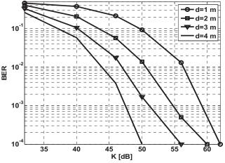
Figure 2. Effect of K on the BER of UMTS receiver for R=600m and for different values of d, and for downlink channel of vehicular test model.
