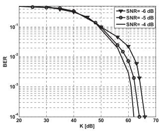
Figure 3: Effect of K on the BER of UMTS receiver for AWGN downlink channel, and for R=600m and d=1m.
