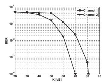
Figure 4. Effect of *K* on the BER of UMTS receiver for multipath fading channels, and for R=600m and d=1m.
