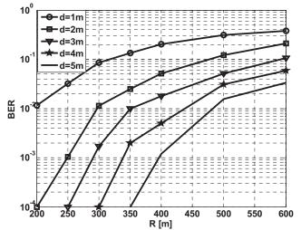
Figure 1. Effect of R on the BER of the UMTS mobile phone receiver for different values of d, and for downlink channel of vehicular test model.
