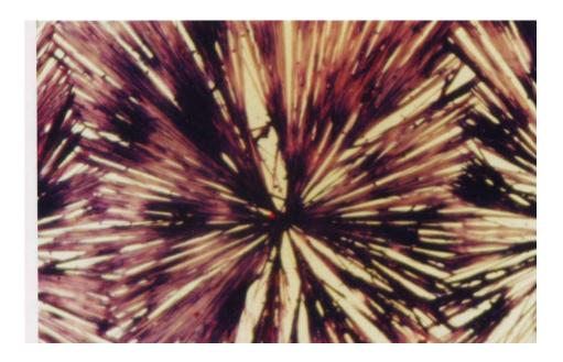
Figure(4):Malts cross-like pattern for Spheralites viewed under polarizing microscope ,the large and small Spherulites are result of crystallization
