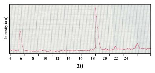
Figure( 5 ):XRD for PCVT thin film at R.T
