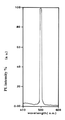
Figure(7):The PL spectrum for PCVT thin film at R.T  $\lambda_{em}$ =504nm , $\lambda_{ex}$ =497nm
