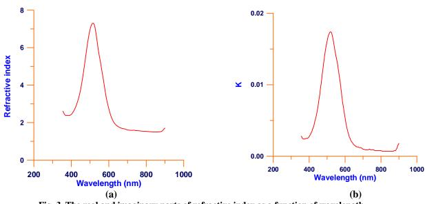
Fig. 3. The real and imaginary parts of refractive index as a function of wavelength.
