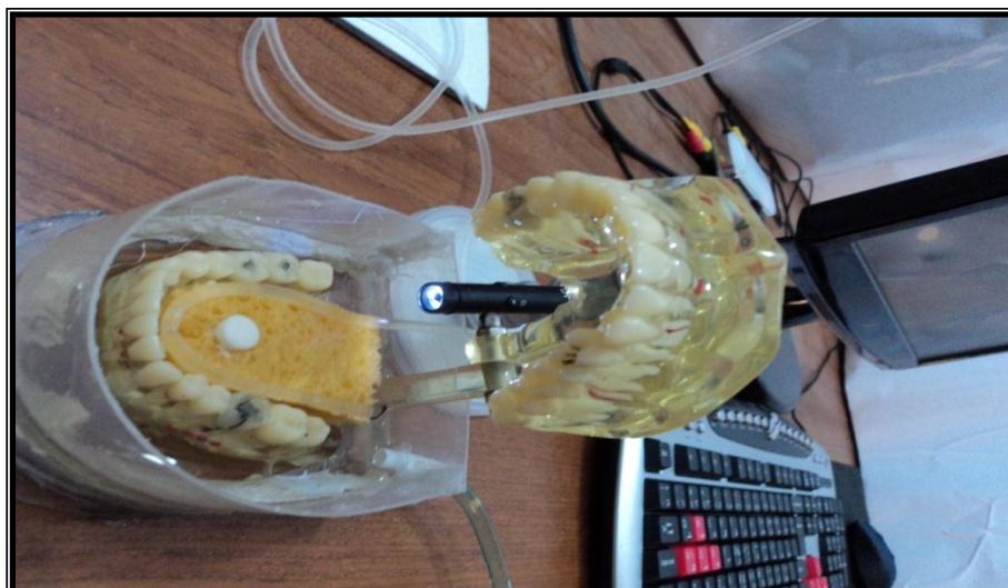
Figure 2. Artificial oral cavity part of MG apparatus
