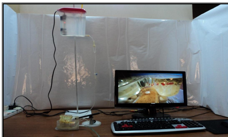
Figure 1. New disintegration apparatus (MG apparatus) for ODTs
