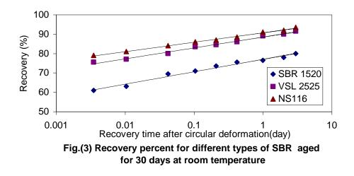
This can be explained by the crosslink densities. A rubber material with higher crosslink density has higher modulus and is stiffer than that with lower one [14]. A rubber material having the higher modulus property will be recovered faster from the deformed shape to the original linear shape than that having the lower modulus.
