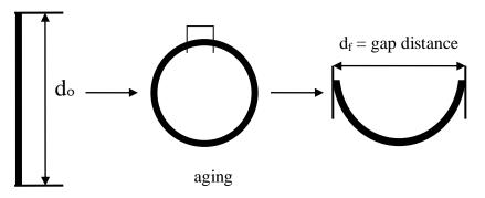
Sketch-2: steps of circular deformation and recovery experiment
