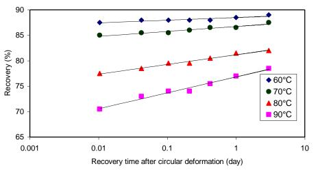
Fig.(5) Recovery percent of NS116 aged at different temp. in circular form versus time after sample release.
