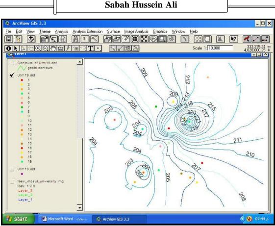
Figure (7): The orthometric heights contour map (1m intervals) of Mosul University
