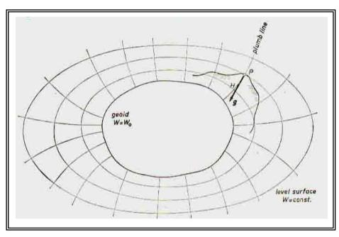
Figure (1): level surface and plumb lines (Ref.7)
