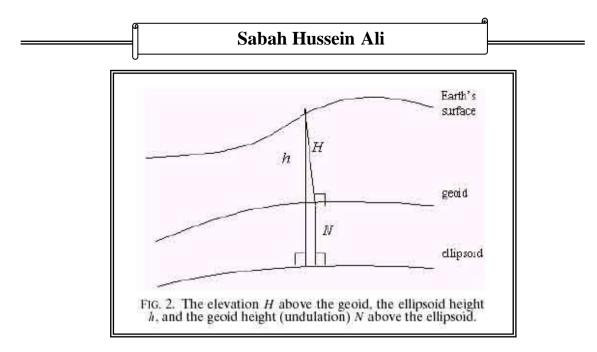
Figure (2): The elevation (H) above the geoid, the ellipsoid height (h), and the geoid height (undulation) (N) above the ellipsoid (3)
