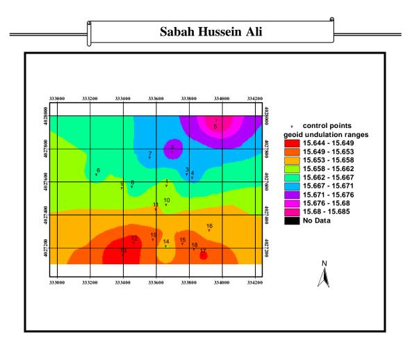
Figure (6): Map of Geoid undulation ranges inside Mosul University campus according to EGM96 global geoid model
