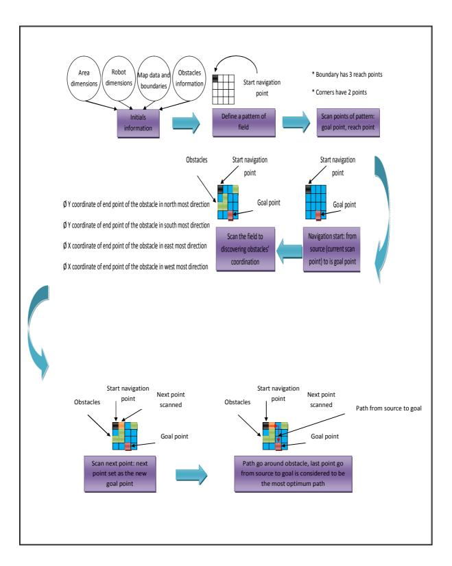
Fig.(2): Block diagram operation of agent (robot) in state space (map)
