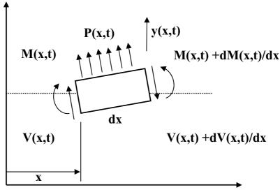
Fig 2. Effect of Forces on the rotating shaft
