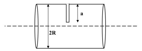
Fig 1. Geometry of a shaft with a transverse crack
