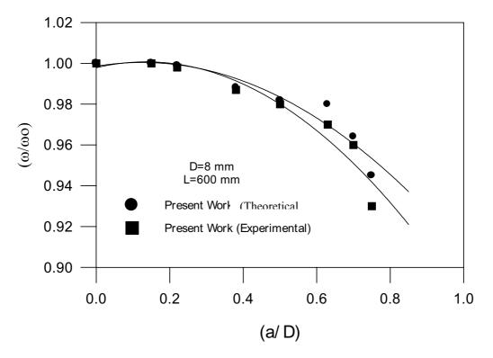
Fig 5.Frequency drop vs crack depth ratio
