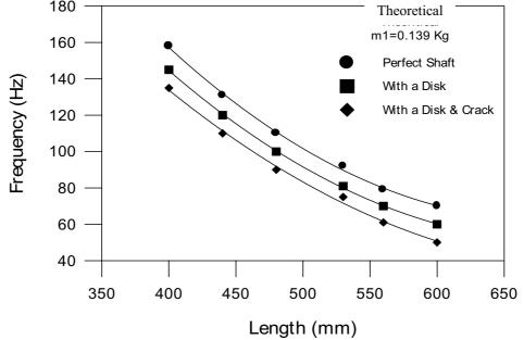
Fig 7.Effect the crack and the load (disk) On the change of frequency (Theoretical)
