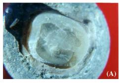
Figure (5A and B): Example of cohesive fracture
