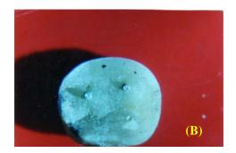
Figure (7A and B): Cohesive fracture with pin group
