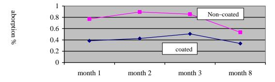
Figure (1): Percentage absorption of coated and non-coated soft liner
