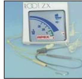
Electronic apex locator device (ROOT ZX) with lip -clip and file holder
