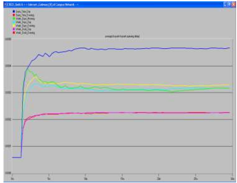
Figure 22: The Average Queuing Delay (Sec) between CISCO Router → Internet_Gateway
