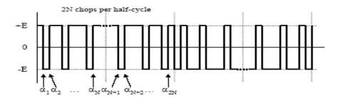
Fig.1: Waveform of a 2-level SHE PWM
