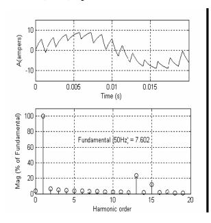
six switching angles circuit in the off-line state.
