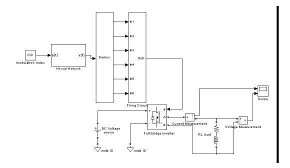
Fig. 4: The Simulink model of full bridge inverter using neural network control with six switching angles
