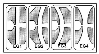
Fig. 2: The wehnelt-anode electrode face shapes of the electron guns EG1, EG2, EG3 and EG4.
