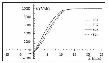
Fig. 3: Comparison between the axial potential distribution of the electron guns EG1, EG2, EG3 and EG4 calculated at ( $V_w = -1 \text{ kV}$  and  $V_A = 10 \text{ kV}$ ).
