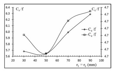
Fig. 11: Comparison of the relative spherical and chromatic aberration coefficients ( $C_s/f$  &  $C_c/f$ ) of the electron gun models as a function of equal values of the wehnelt and anode face curvature ( $r_1=r_2$ ), calculated at  $V_W=-1kV$  and  $V_A=10kV$ .
