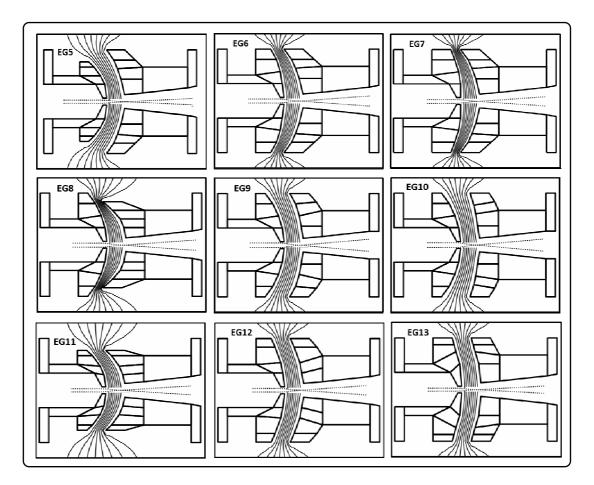
Fig. 7: The equipotential lines (continuous lines) and the electron trajectories (dotted lines) due to the electron guns EG5, EG6, EG7, EG8, EG9, EG10, EG11, EG12 and EG13, calculated at  $V_w$ = -1 kV and  $V_A$ =10 kV.
