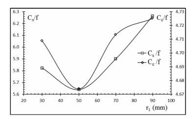
Fig. 9: Comparison of the relative spherical and chromatic aberration coefficients ( $C_s/f \& C_c/f$ ) of the electron gun models as a function of radius of the wehnelt face curvature  $r_1$  at constant anode face curvature ( $r_2$ =50 mm), calculated at  $V_W$ =-1kV and  $V_A$ =10kV.
