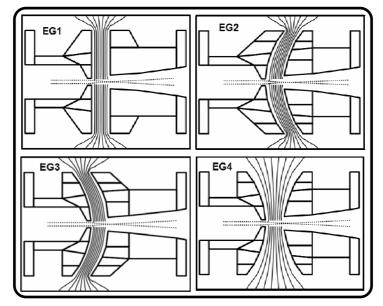
Fig. 4 : The equipotential lines (continuous lines) and the electron trajectories (dotted lines) due to the electron guns EG1, EG2, EG3 and EG4, calculated at  $V_w$ = -1 kV and  $V_A$ =10 kV.
