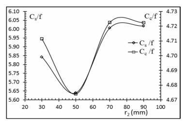
Fig. 10: Comparison of the relative spherical and chromatic aberration coefficients ( $C_s/f \& C_c/f$ ) of the electron gun models as a function of radius of the anode face curvature  $r_2$  at constant wehnelt face curvature ( $r_1$ =50 mm), calculated at  $V_W$ =-1kV and  $V_A$ =10kV.
