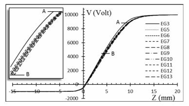
Fig. 6 : Comparison between the axial potential distribution of the electron gun EG3 with those of EG5, EG6, EG7, EG8, EG9, EG10, EG11, EG12 and EG13 calculated at  $V_w = -1$  kV and  $V_A = 10$  kV.
