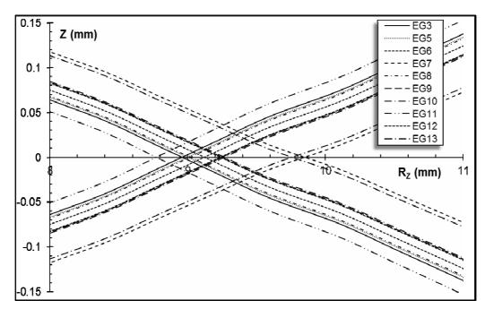
Fig. 8: The paraxial electron beam trajectories at the cross-over points of the electron models EG3, EG5, EG6, EG7, EG8, EG9, EG10, EG11, EG12 and EG13, calculated at  $V_w = -1$  kV and  $V_A = 10$  kV.
