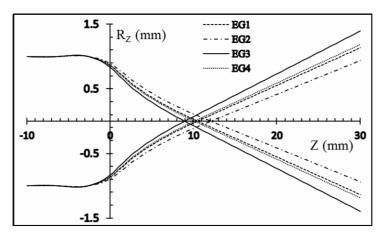
Fig. 5: Comparison between the paraxial ray trajectories  $R_z$  of the electron beam in the electron guns EG1, EG2, EG3 and EG4, calculated at  $V_w = -1 \text{ kV } \& V_A = 10 \text{ kV}$ .
