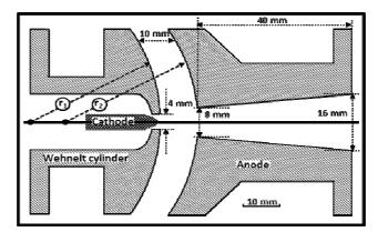
Fig. 1: Cross section of the electron gun electrodes with its geometrical parameters
