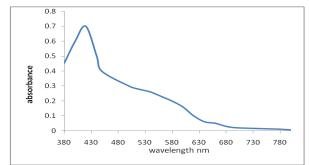
Figure(2) the absorbance spectra for the alizarin red (S) vs. DDW
