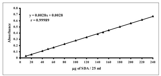
Fig. 1: Calibration graph of SDA determination.
