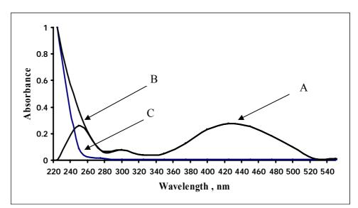
Fig. 2. :Absorption spectra of 100 μg / 25 ml SDA treated according to the recommended procedure and measured against (A) reagent blank, (B) distilled water and (C) reagent blank measured against distilled water
