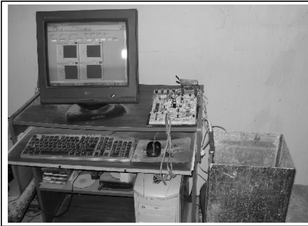
Figure (1): The picture of the experimental for the real-time control of temperature of a heating
