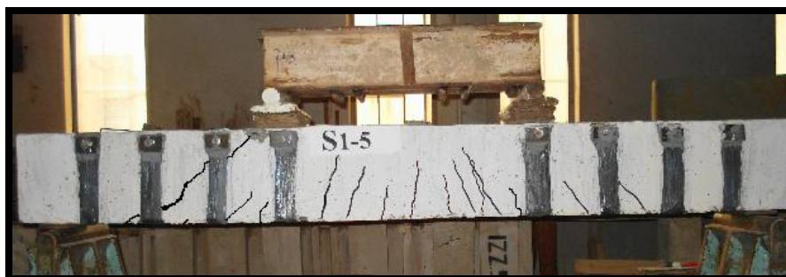
Figure 10: Crack pattern at ultimate failure of specimen S1-5
