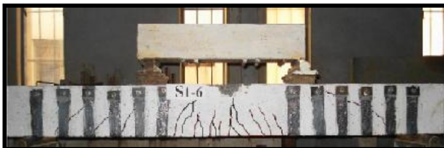
Figure 11: Crack pattern at ultimate failure of specimen S1-6
