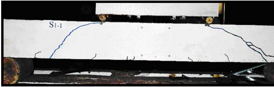
Figure 5: Beam specimen S1-1 as a control beam with steel stirrups (a/d=3)
