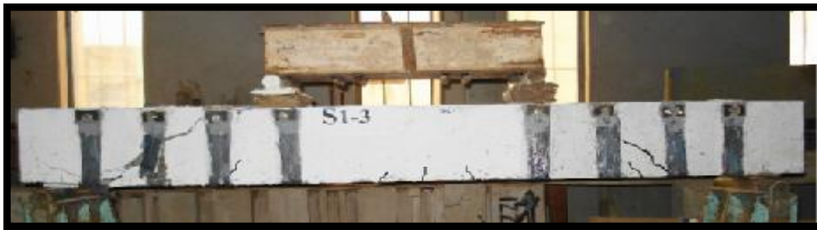
Figure 7: Crack pattern at ultimate failure of specimen S1-3
