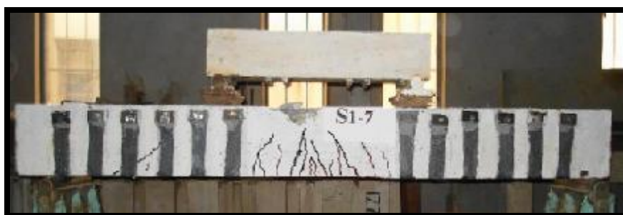
Figure 12: Crack pattern at ultimate failure of specimen S1-7
