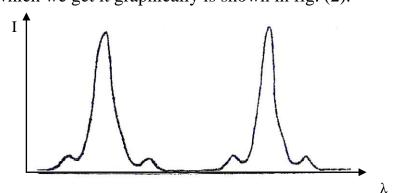
Fig. (2): The spectral line profile of hollow cathode discharge tube, Cr ( $\lambda$ = 425.4 nm)
