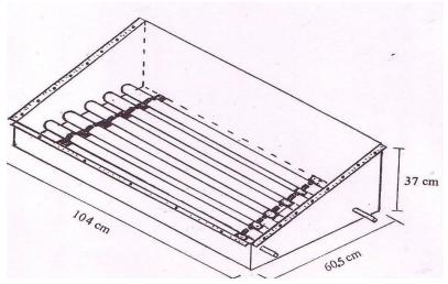
Fig. (1): Schematic diagram of the solar still.
