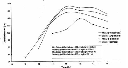
Fig. (5): Comparison of the productivity between painted and unpainted solar stills using chemical converters of M3g.
