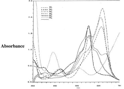
Fig. (2): Absorption spectra of individual dyes (M1-M7).
