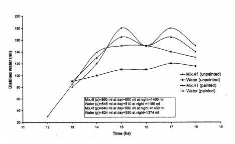
Fig. (6): Comparison of the productivity between painted and unpainted solar stills using chemical converters of M4f.
