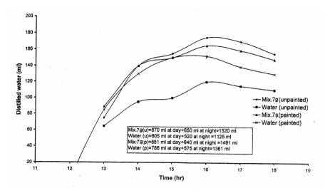
Fig. (7): Comparison of the productivity between painted and unpainted solar stills using chemical converters of M7g.
