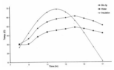
Fig. (4a):Thermal performance plots of optimum mixture M3g.
