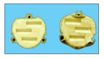
Figure (3): Mould Used in Preparing Tensile Test Specimen.
