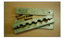
Figure (2): Split Metal Mould for preparing acrylic cylinder.
