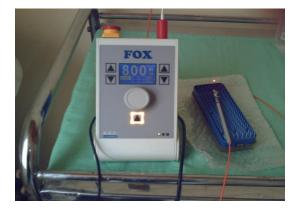
Figure (3): Diode laser 1064nm, Fox.
