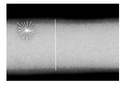
Figure (6): Measuring the area of irregular porosity in the radiographic image by Dimax program
