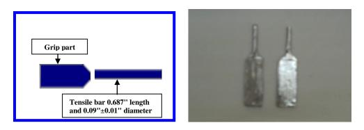
Figure (2): Illustrates the grip part and the tensile bar of the second group
