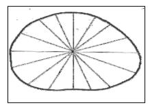
Figure (5): Record measurements to the nearest point, from the edge of the area to the center of the circle every 20 degrees. (HGIC,2005)
