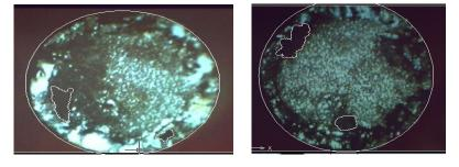
Figure (7): Auto CAD drawings on the cross section and around the porosities in the fracture's photograph
