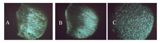
Figure (8): Microscopic view of the treated cross sections, A- Polished surface, B- Laser treated, C- Sandblasted surface
