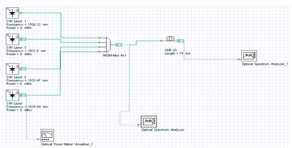
Fig (8): four unequally-spaced frequencies (1530.33, 1531.90, 1533.47, and 1535.04) nm without FWM.
