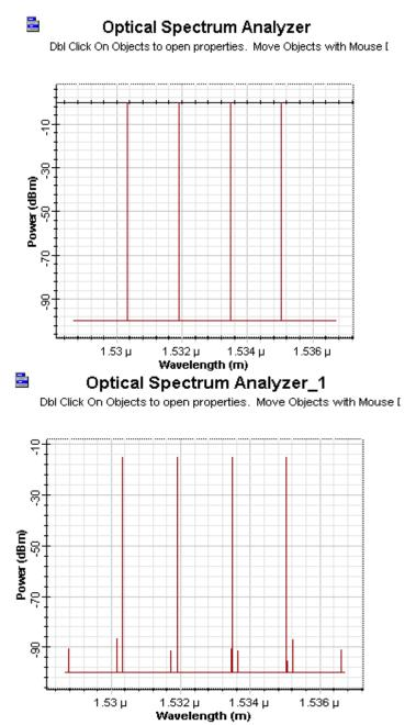
Fig. (11): with 40Gbit/s, the output with FWM is shown
