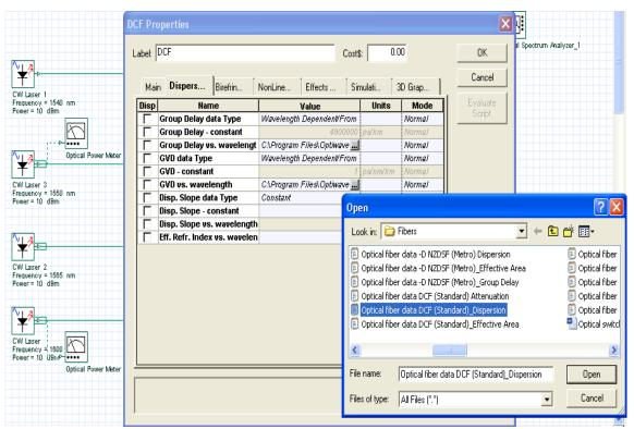
Fig. (12): optical fiber data DCF\_ Dispersion and optical fiber data DCF\_ Attenuation are loaded from the library of Optisystem 4.0
