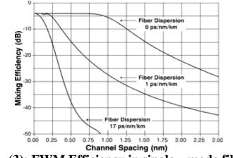
Fig. (3): FWM Efficiency in single – mode fibers
