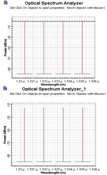
Fig. (10, A): the input and output of four unequally spaced Fig. (10, B): The output of the system, not Frequencies (1530.33, 1531.90, 1533.47, and 1535.04) nm affected by FWM
