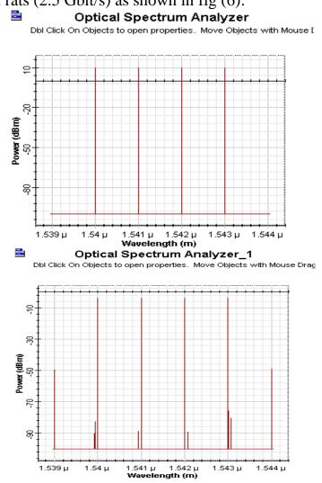
Fig .(6, A): shows the input four signals to the SMF Figure 6B shows the four signals at the output of SMF Fiber Fiber, affected by FWM.
