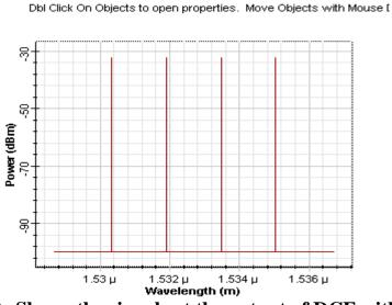
Fig. (13, C): Shows the signals at the output of DCF without FWM
