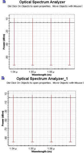
Fig. (7, A): Four channels at the input of the fiber Fig (7B) Four channels at the output of the fiber,
