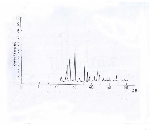
Fig(A-2):X-ray diffraction of (Bi<sub>2</sub>Ba<sub>2</sub>Ca<sub>2</sub>Cu<sub>3</sub>O<sub>7</sub>-δ)at(830)C°
