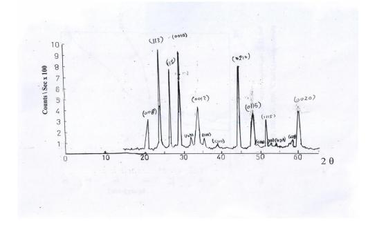
Fig(A-4):X-ray diffraction of(Bi<sub>2</sub>Ba<sub>2</sub>Ca<sub>2</sub>Cu<sub>3</sub>O<sub>7</sub>-δ)at(890)C°
