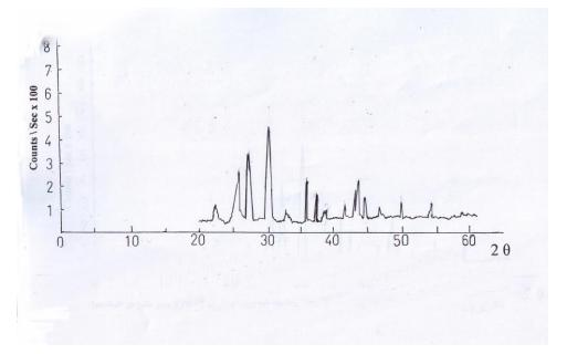
Fig(A-1):X-ray diffraction of(Bi<sub>2</sub>Ba<sub>2</sub>Ca<sub>2</sub>Cu<sub>3</sub>O<sub>7</sub>-δ)at(790)C°
