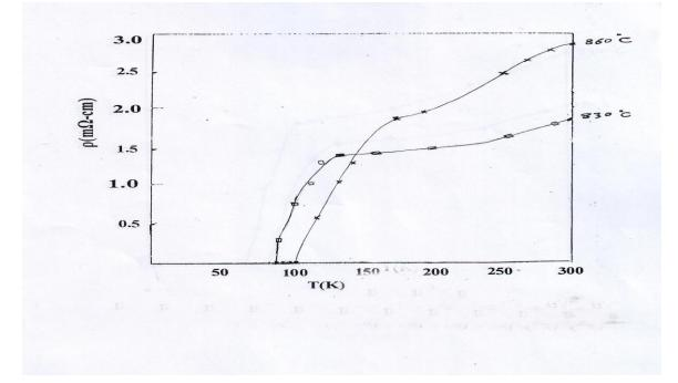
Fig(B-1):Variation of resistively with temperature for(Bi<sub>2</sub>Ba<sub>2</sub>Ca<sub>2</sub>Cu<sub>3</sub>O<sub>7</sub>- $\delta$ ) at(790,890)C°
