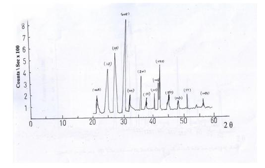
Fig(A-3)X-ray diffraction of  $(Bi_2Ba_2Ca_2Cu_3O_7-\delta)at(860)C^{\circ}$
