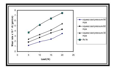
Figure (5) Effect of squeeze cast pressure on wear rate , under different load for the Al- alloy and composites, constant sliding speed (3.08) m/sec.
