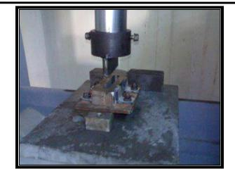
Figure (2) the punch and die used in squeeze casting
