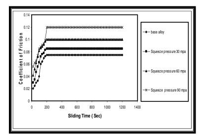
Figure (9) Coefficient of friction the base alloy and composites which casts under different squeeze pressure in function of sliding time. Load 10 N,sliding speed 4.7 m/sec
