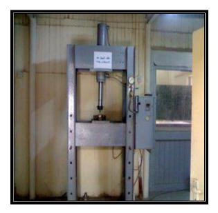
Figure (1) the hydraulic press used for squeeze casting .
