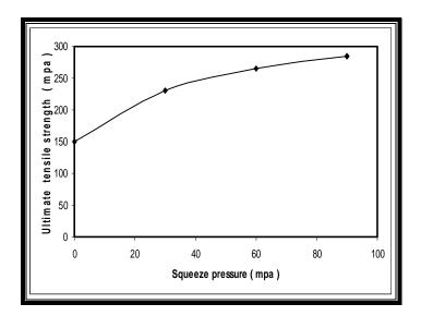
Figure (11). Effect of squeeze pressure on ultimate tensile strength
