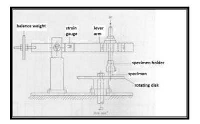
Figure (3) Wear test apparatus
