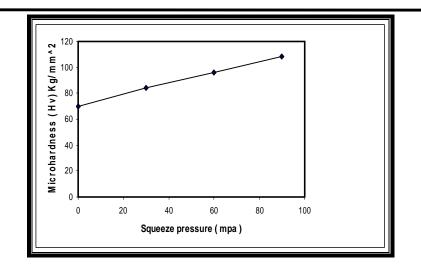
Figure (12) Effect of squeeze pressure on microhardness
