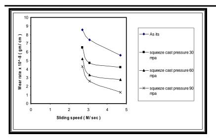
Figure (6) Effect of squeeze pressure on wear rate under Different sliding speed for the base Al- alloy and composite, constant load 10 N.
