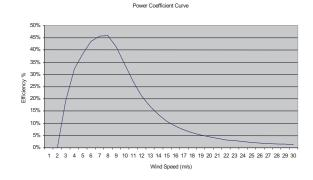
Fig. 4 Power Coefficient, Cp for 15kW Proven wind turbine
