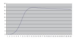
Fig. 3 Power curve for 15kW Proven wind turbine
