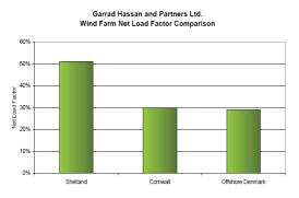
Fig. 1 Comparison between wind energy resource in Shetland, Cornwall (UK) and Denmark
