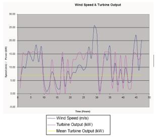
Fig. 5 Time-series wind speed and the corresponding simulated wind turbine power output
