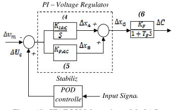
Figure (4): STATCOM dynamic model of AC voltage regulator and POD stabilizer
