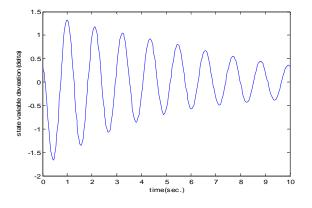
Figure (5): Dynamic response for  $\Delta \delta$  without controller
