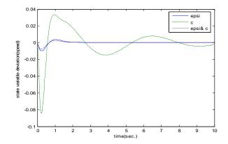
Figure (12): Dynamic response for  $\Delta \omega$  with proposed schemes (scheme 2, 3 and 5).
