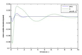
Figure (10): Dynamic response for  $\Delta \omega$  with proposed schemes (scheme 1, 3 and 4).
