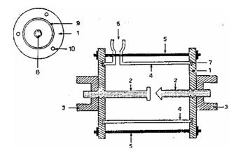
Fig. 2: Schematic diagram for the test cell1. Obonite base.2. Brase electrode.3. Plexy glass.4. Glass test cell envelope.5. Steel fitting rods.6. Filling port.7. Gasget.8. Electrode fitting hole.9. Test cell setting grove.10. Rod fitting hole.
