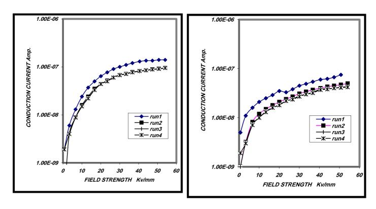
Effect of electrical purification on the current growth in n-octane & n-pentane respectively.
