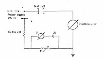
Fig. 3: the Schematic diagram of experimental circuit. G, electronic galvanometer ,  $\mu$  standard cell , R , standard resistor , r available resistance box .
