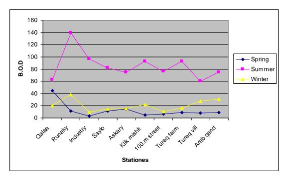
Figure (5) Biochemical Oxygen Demand in the Erbil waste water channels during the three studied periods.
